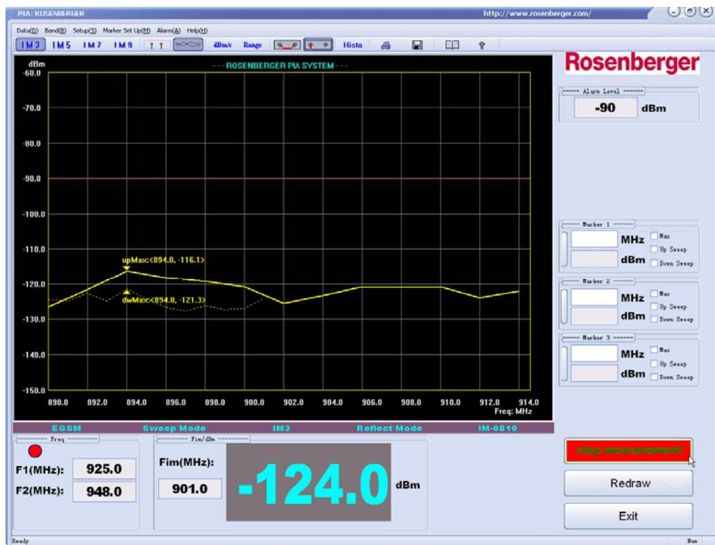
Fig 2-5 Sweep measurement result
