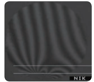
1,000 μm diameter fiber Interference microscope image 1 stripe = 0.01°
