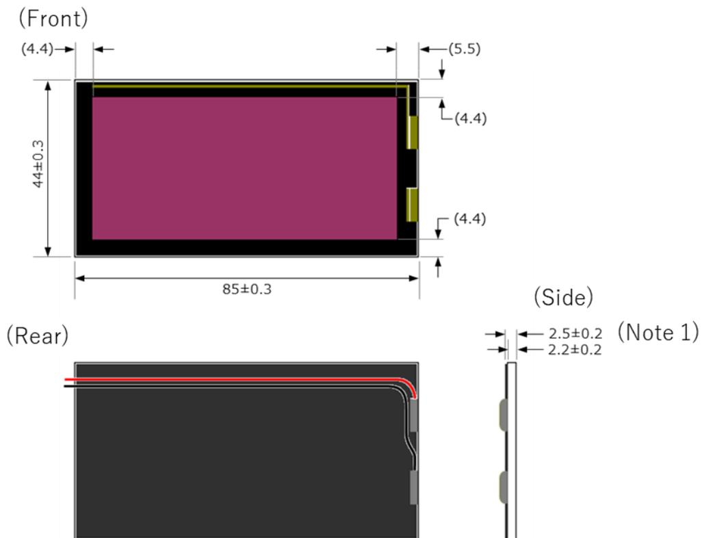
The figures show the dimensions of the main unit of the solar cell.
