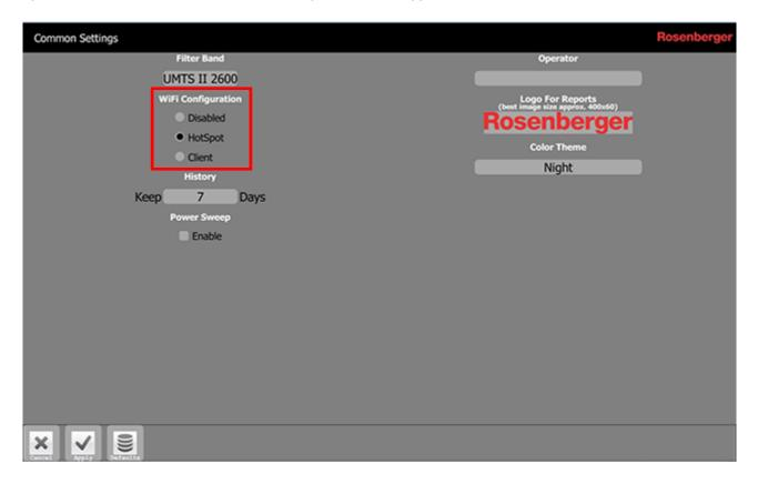
Open the WiFi connections screen on your tablet and connect with the network entitiled with the SSID shown on the PIM Site Analyzer  $\alpha$ . You will be prompted to input the password also shown on your device's screen.
