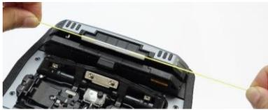
\* Apply tension to the fiber until heater clamps hold it.
