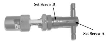
QJST is color coded to indicate cable size and is removed for flooded cable jacket stripping
