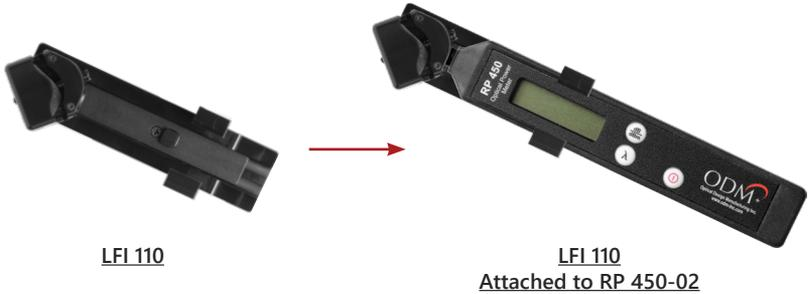
To use the LFI 110 accessory with the RP 450-02, remove the adapter on the RP 450-02 power meter and slide the two units together until they snap firmly in place (see pictures above). To separate the units, grasp the LFI 110 firmly with the thumb and forefinger and pull the device away from the power meter.
