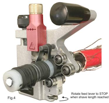
Shaving operation using the winding pin. Note the direction of the semi-con strip around the pin.
