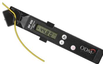
The 2kHz tone output of the DLS 360 can be recognized through the fiber jacket when a Live Fiber Identifier is used.
