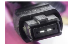
MTP® 12 fibers female with OCTO fiber assignment
